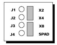
Figure 2 --- Factory default jumper configuration
